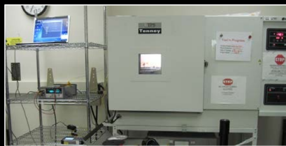
White Light LED Testing in Environmental Chamber
