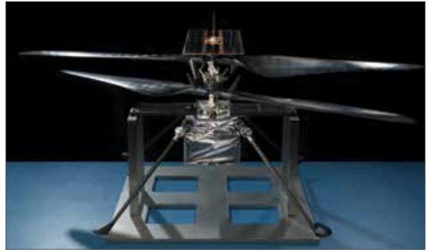
► The finalized Mars Helicopter Flight Model.
