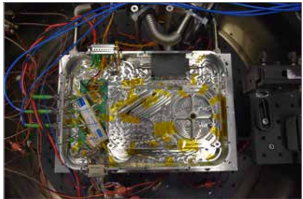
► GSFC in-house power amplifier assembly that meets the LISA requirements.
