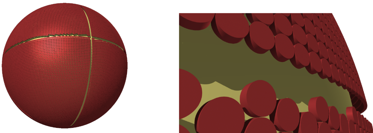
Figure 25. Fully covered 100 m diameter spherical asteroid. An enlarged view of a small section is given on the right. The small cylinders are just a little larger than the implemented detector setup. For technical reasons the sphere had to be covered in 8 identical sections.
