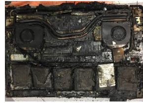
(b) Thermal runaway propagation to all battery cells.
