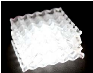
Figure 2 Tortuosity substrates produced with waveguide sheets
