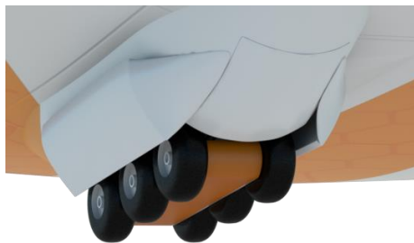
Fig. 12 Illustration of pod gear concept with toboggan.
