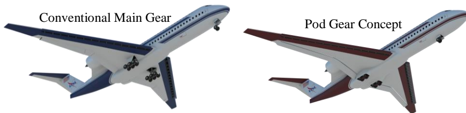
Fig. 11 Comparison between conventional (upper) and pod (lower) landing gear.
