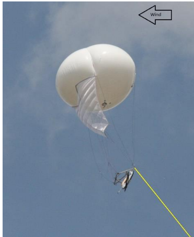
Fig. 8 Aerostat balloon supporting Woodstock with tether highlighted and wind direction indicated.
