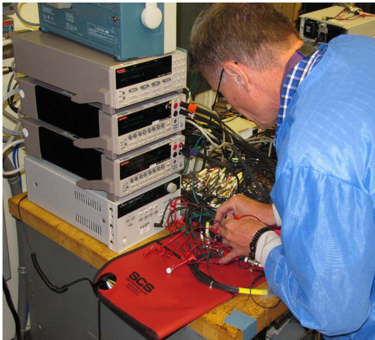
Figure 6: Equipment stack outside cave, and control samples on ESD mat.
