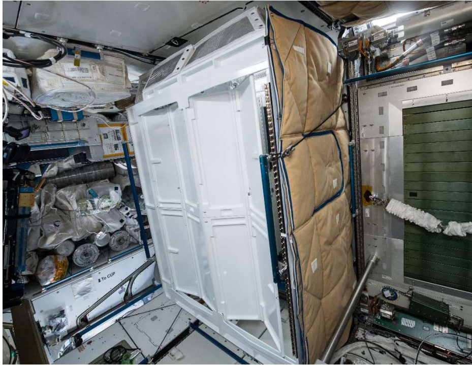
Figure 7. Toilet Stall Deployed on ISS.
