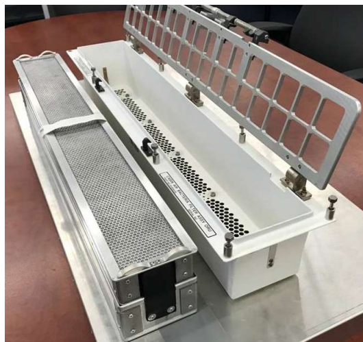
Figure 2. Siloxane and HEPA Filter Flight Hardware.
