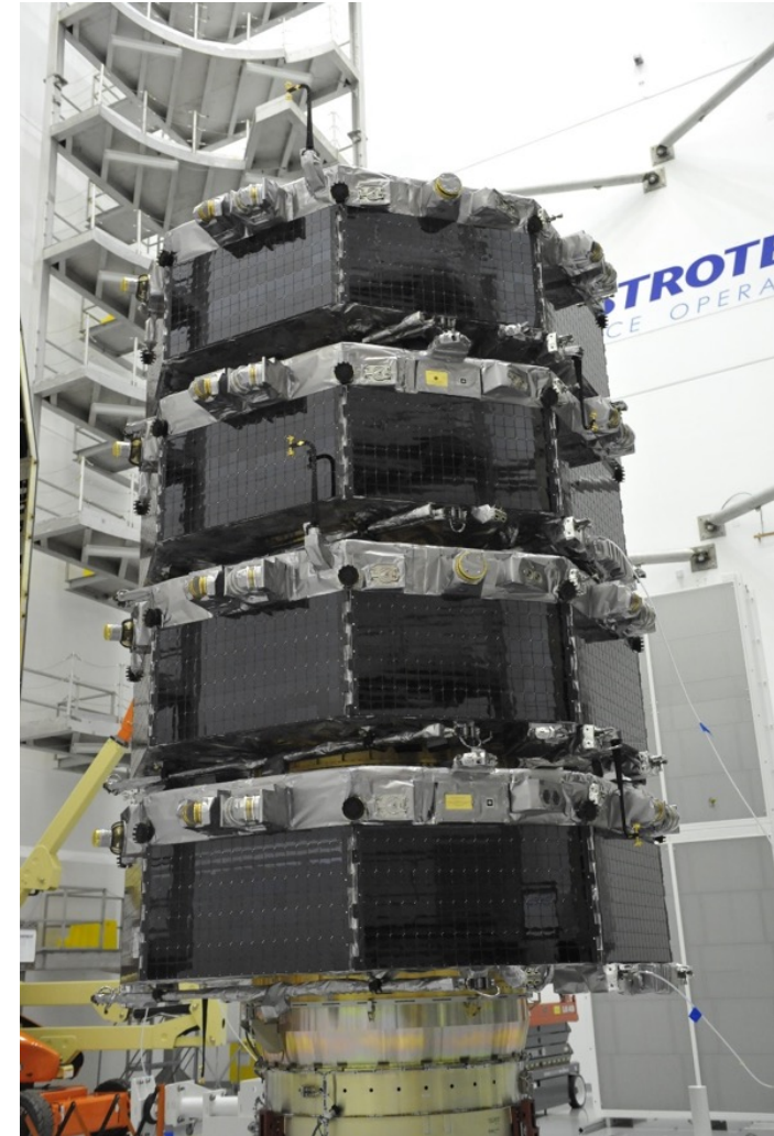
Four Stacked MMS Spacecraft
