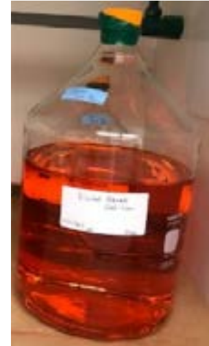
Figure 10. Samples being tested by complete immersion in the diluted ECLSS solution.
