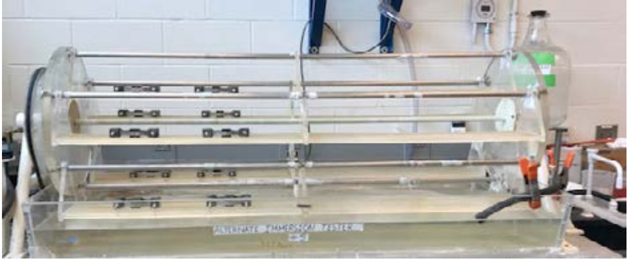
Figure 12. Samples being tested by alternate immersion in 3.5% NaCl solution.
