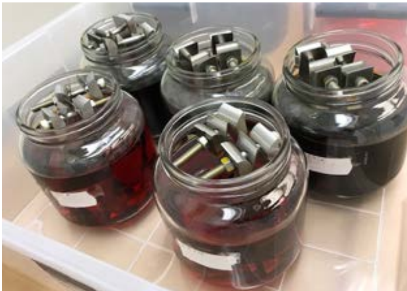
Figure 11. Samples being tested by complete immersion in the concentrated ECLSS solution.
