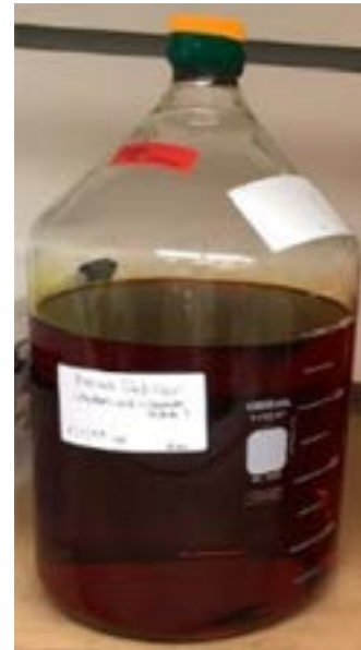
Figure 11. Samples being tested by complete immersion in the concentrated ECLSS solution.
