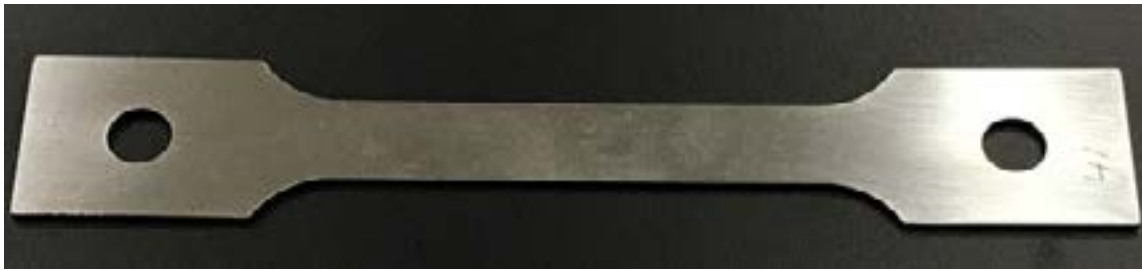
Figure 2. View of representative Elgiloy stress corrosion specimen as received.
