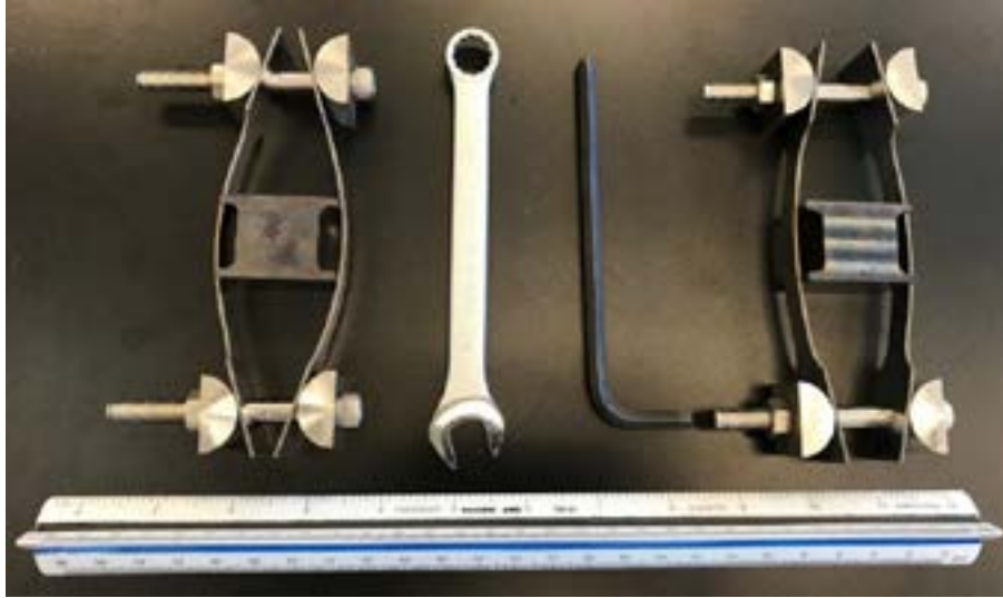
Figure 7. Tools to load beam specimens and representative assembled samples.
