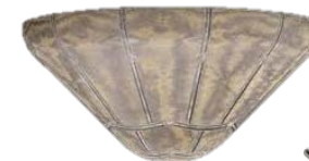
Tiled HEEET Engineering Test Unit
