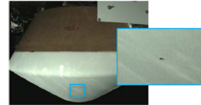
Stardust -> OSIRIS-REx (with Micro-meteoroid damage)
