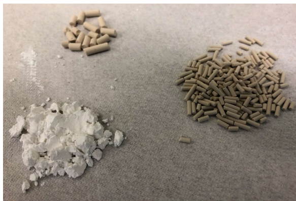
Figure 8. Zeolite 13X in three forms.
