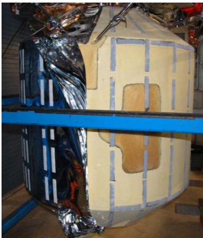
LB-MLI on 4' diameter tank
