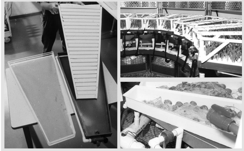
Figure 9. The BPC hydroponic trays. a) Left: Original PVC tray with plant support insert and germination cover shown; b) Upper Right: Original PVC trays in the BPC with young wheat plants; c) Lower Right: BPC trays, vacuum-formed from ABS sheets containing potato tubers (potato tray tops removed). Credits: NASA
