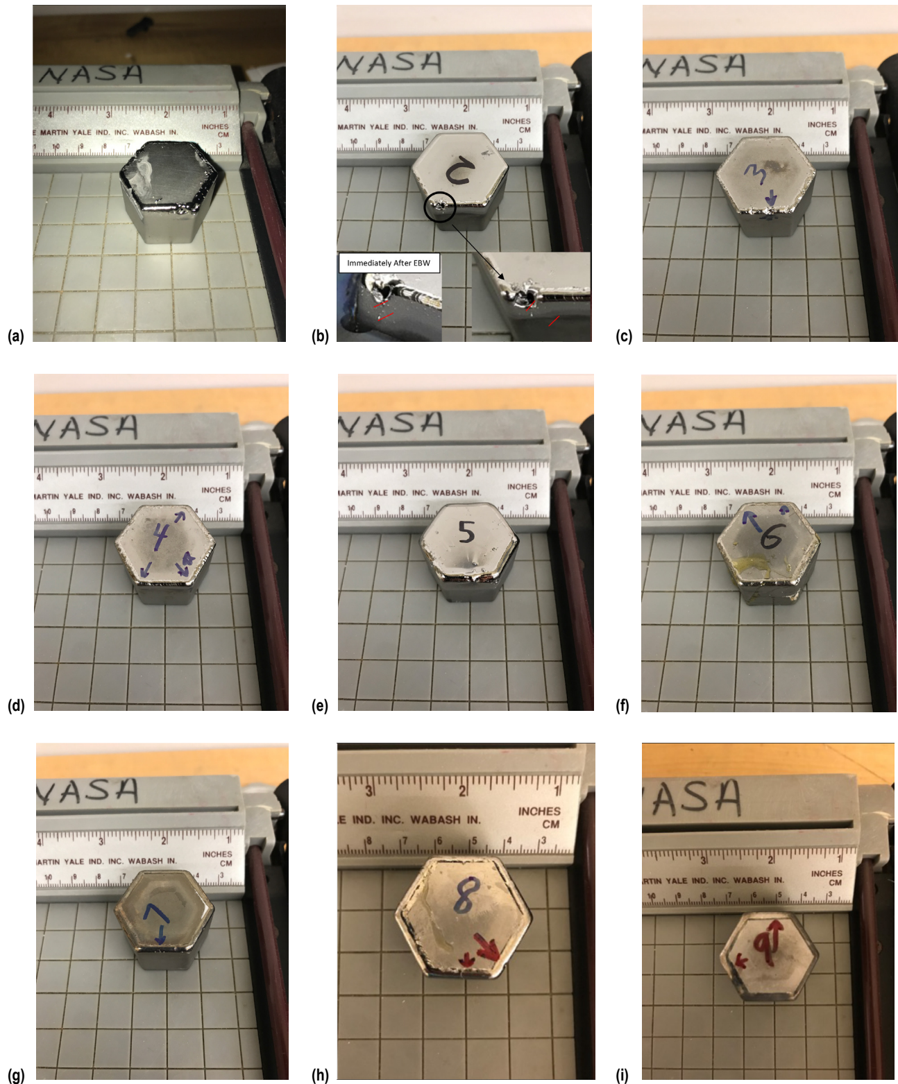
Figure 6. Images of all nine pure tungsten hex can samples: (a) EBW_Hex1, (b) EBW_Hex2, (c) EBW_Hex3, (d) EBW_Hex4, (e) EBW_Hex5, (f) EBW_Hex6, (g) EBW_Hex7, (h) EBW_Hex8, and (i) EBW_Hex9.
