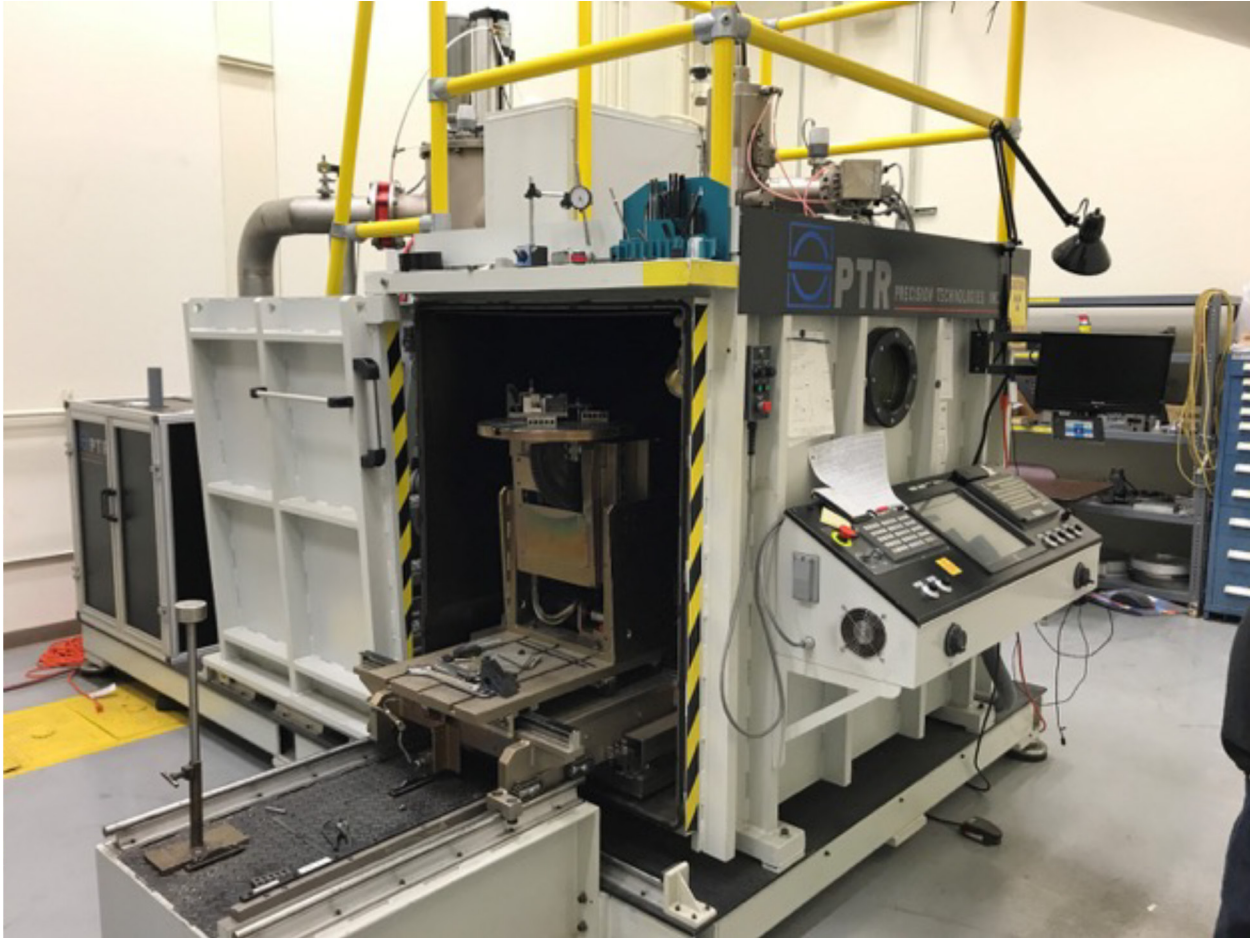
Figure 10. EBW machine used to weld both pure tungsten plates and pure tungsten hex cans.
