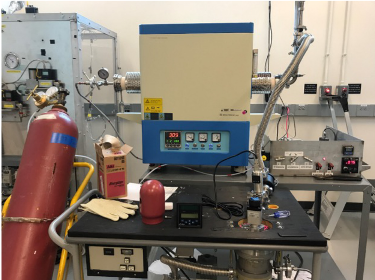
Figure 2. Oven used for PWHT of all pure tungsten hex cans.
