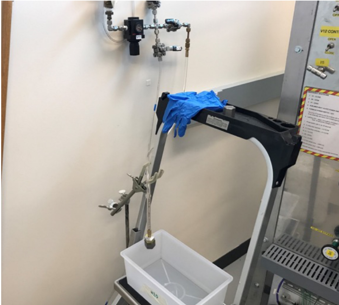
Figure 4. Pressure test setup with EBW_Hex8 attached to the pressure hose and aluminum hex fitting.
