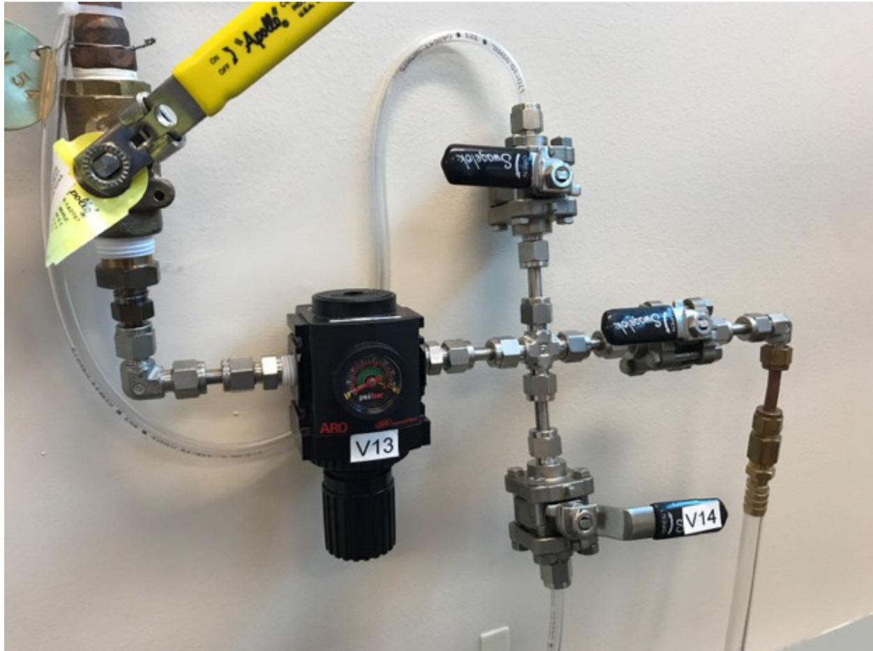
Figure 3. Regulator setup for pressure testing of the pure tungsten hex cans.
