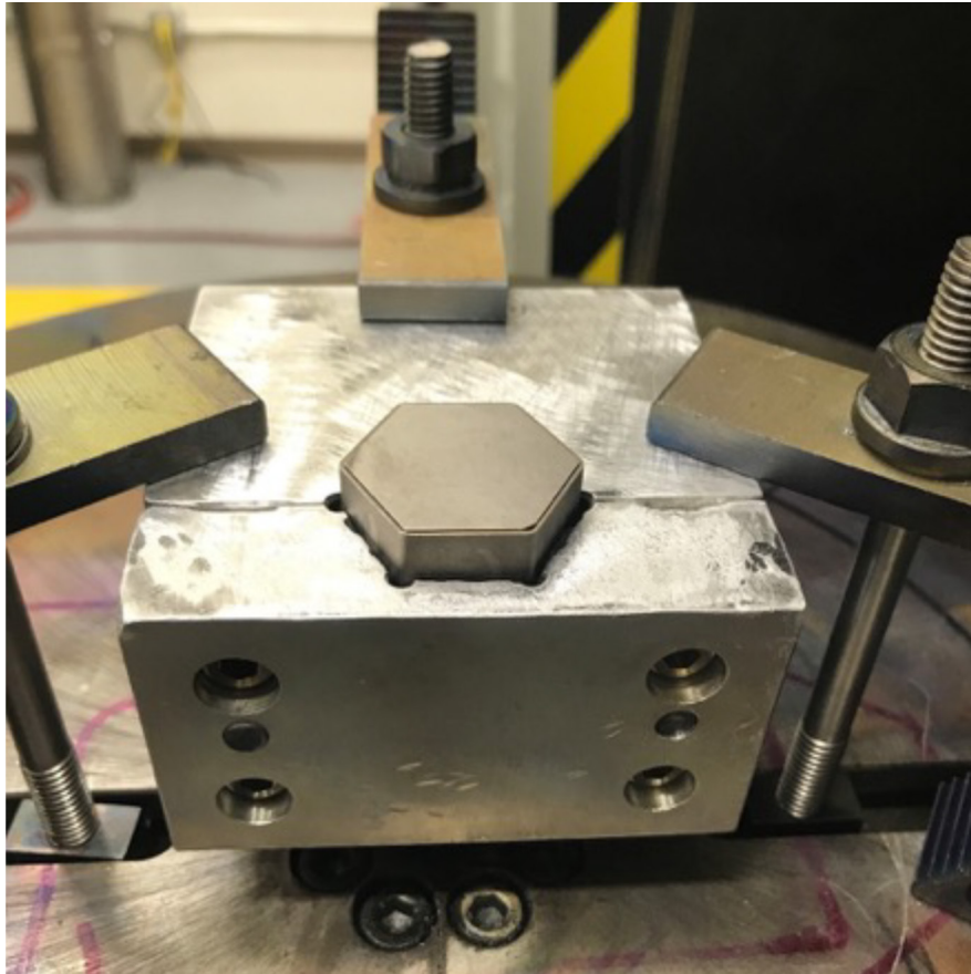
Figure 9. Weld fixture (with EBW_Hex6 in place prior to welding).
