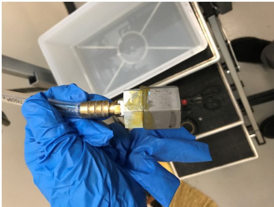
Figure 12. Pressure hose and aluminum hex fitting designed to pressurize the EBW tungsten weld. Polymer binder applied using a heat gun to make the interface leak tight.
