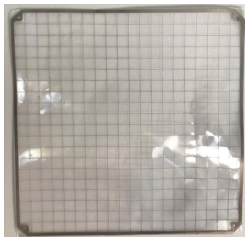
Fig. 10. Embedded Mesh Lens After Dissolving Tool.
