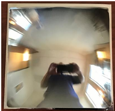
Fig. 5. Nickel Electroform Replica of Master Tool.
