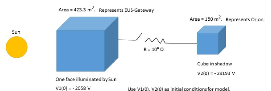
$C_{11}=1.12$ e-9 F,  $C_{22}=7.81$ e-10 F,  $C_{12}=-6.07$ e-10 F,  $C_{21}=-6.30$ e-10 F.  $\Rightarrow C_{mutual}=7.414$ e-10 F.
