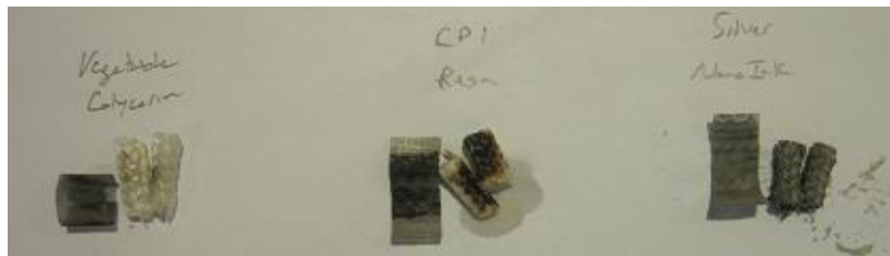
Figure 3. Photographs of wicks after testing of three different fluids.
