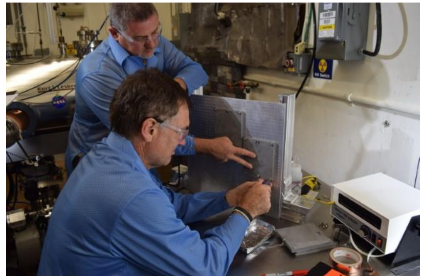
Preparing sample plate with live propellant
