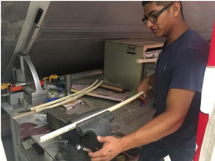
Bending CPVC to create hatches
