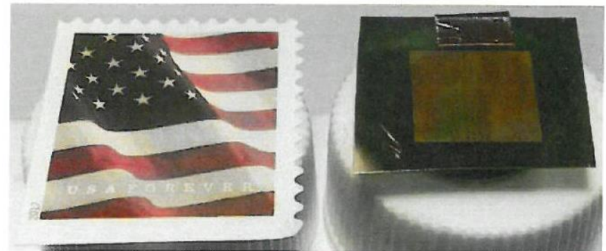
UTSI's μSTAMP electro spray thruster
