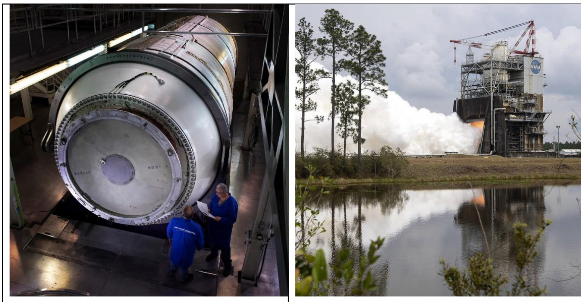
Figure 6: EM-1 SRB motor segment, left, and February 2019 RS-25 test firing, right
