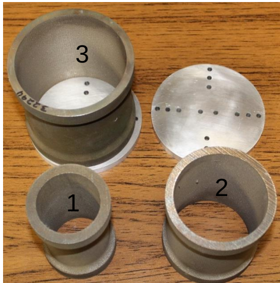
Cylinder 1: 2" diameter x 1/8" wall Cylinder 2: 3" diameter x 1/8" wall Cylinder 3: 4" diameter x 1/8" wall
