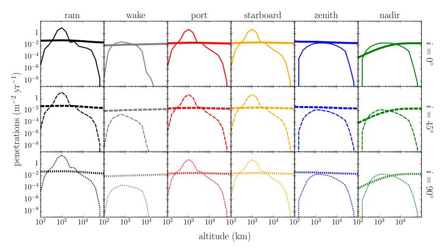
Meteoroids dominate the one millimeter penetrating flux at altitudes below 250 km and above 4000 km.
