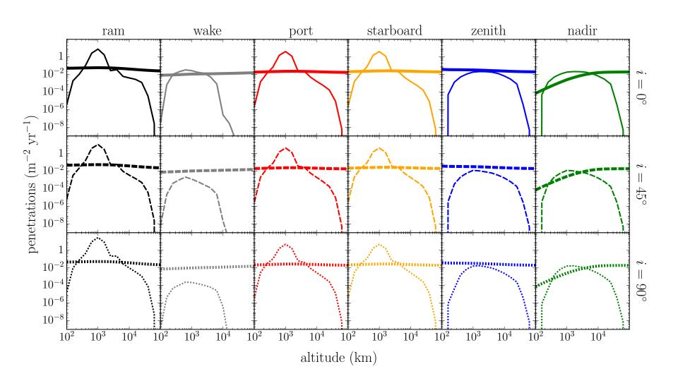
Meteoroid penetrating flux varies by only a factor of a few over all surfaces and altitudes; that of orbital debris spans several orders of magnitude.
