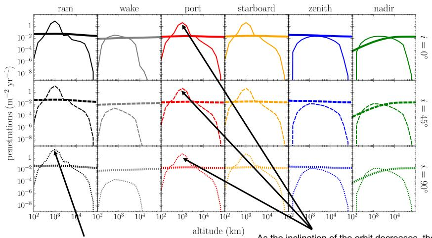
At 1000 km and 90° inclination, the number of debris penetrations is almost 500x that of meteoroids.
