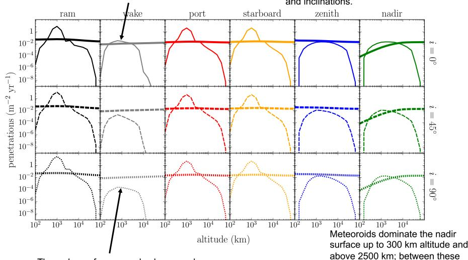
The wake surface may also be a good place for meteoroid detector if the vehicle is in an orbit with inclination near 90°
