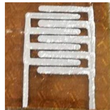
Al-Fe 2 O 3 electrode CO 2 sensor
