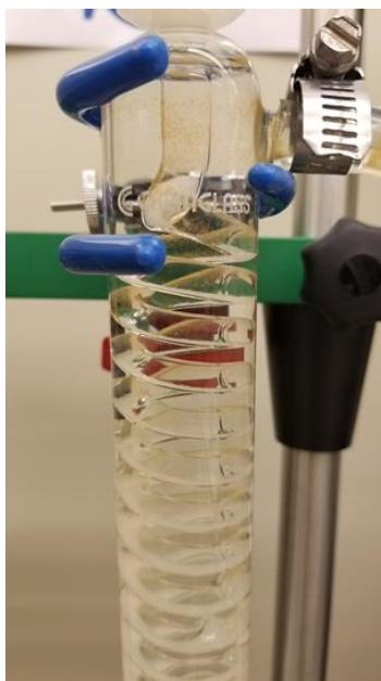
Figure 11. Crystals deposited in the heat exchanger.
