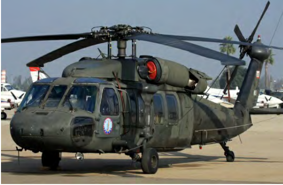
Figure 1 Sikorsky UH-60A Blackhawk helicopter on apron. Note flexible blades.
