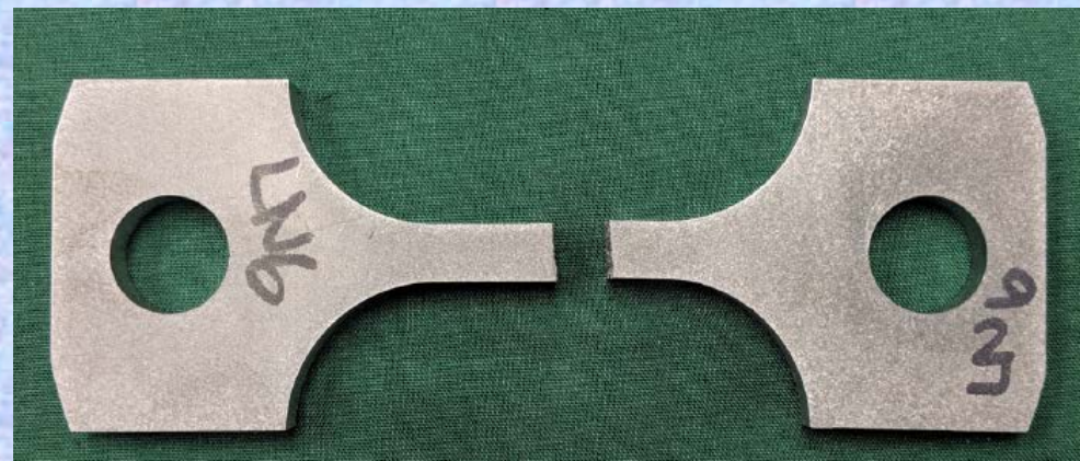
Broken Specimen in gage section
