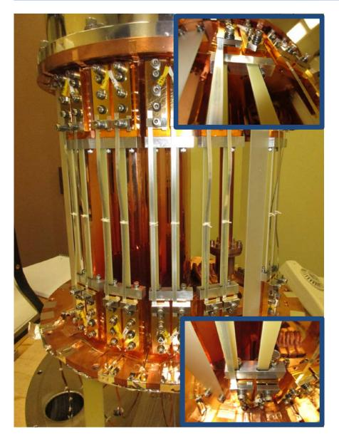
Strongbacks made from G10 installed behind each tape
