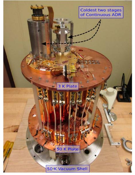
10 current leads needed to run the 4 CADR stages and the superconducting heat switch between Stages 1 and 2
