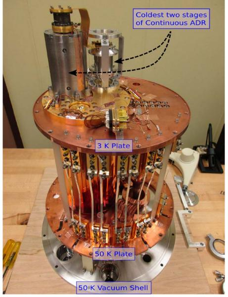
A cryostat was built to contain a 4-Stage Continuous Adiabatic Demagnetization Refrigerator (CADR).
