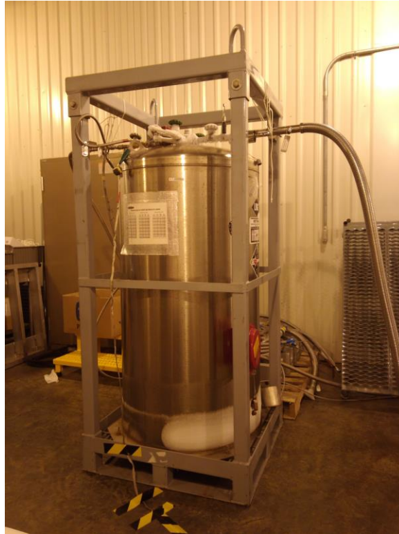
Figure 6. LNG Microfueler, flowing liquid methane to the RRM3 payload
