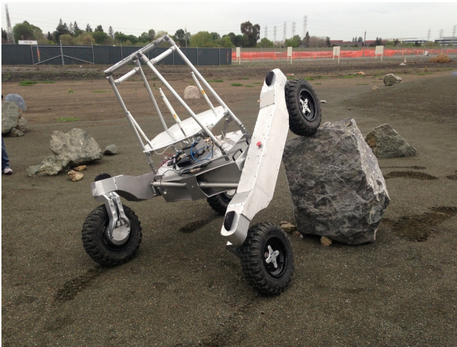
Figure 13: KRex2 exercising the differencing bar to maintain terrain contact for all wheels.
