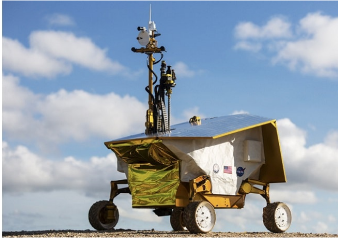
(a) The Resource Prospector (RP) robot is capable of independently steering each of its wheels. Additionally, each wheel can be raised and lowered independently, permitting the robot to “walk” out of sand traps.
