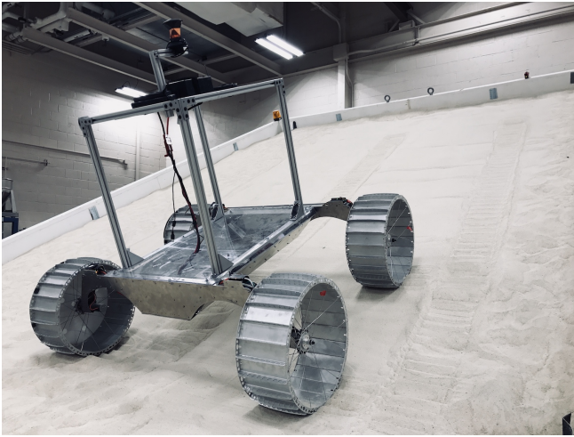
Figure 15: A picture of the RP Lunar mass equivalent rover at the SLOPElab in NASA GRC.
