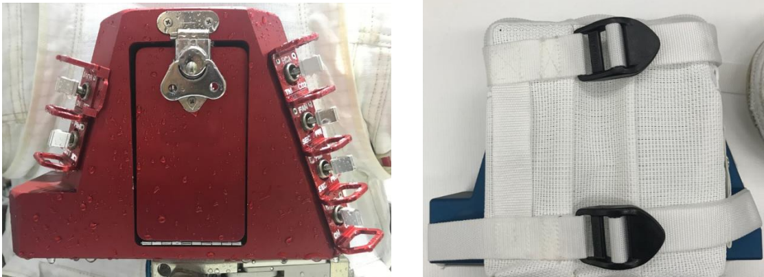
Figure 2. The NBL DCU mock-up is a volumetric representation with the primary purpose of helping to achieve a neutral buoyancy in the water column. The mock-up on the left (red) is the high fidelity DCU mock-up with representation switches and switch guards. The mock-up on the right (blue) is the low fidelity DCU mock-up. It is a simpler, heavier version of the DCU mock-up. It is shown with a custom weight pack attached to assist with getting more weight on the suit.
