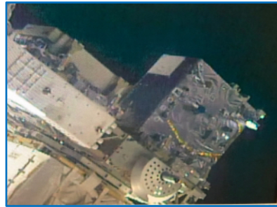
RRM3 Fuel Transfer Module (FTM) on the International Space Station (ISS).
