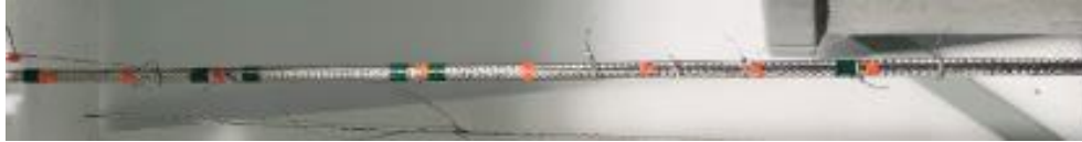
Figure 1. EDU flex-hose with imperfections marked in green. Image credit: Brian Nufer, NIFS mentor.
