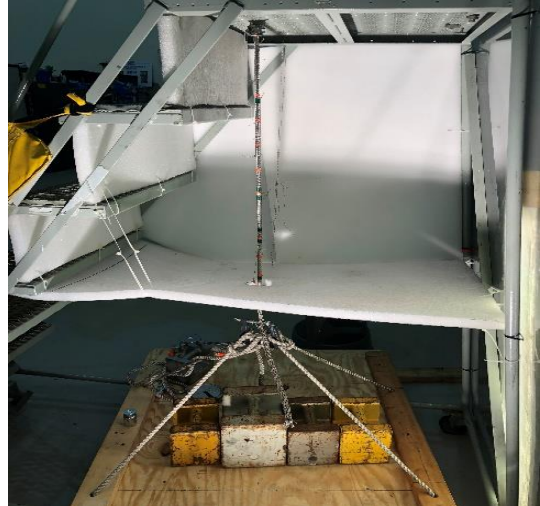
Figure 3. Maximum load configuration. Image credit: Brian Nufer, NIFS mentor.
