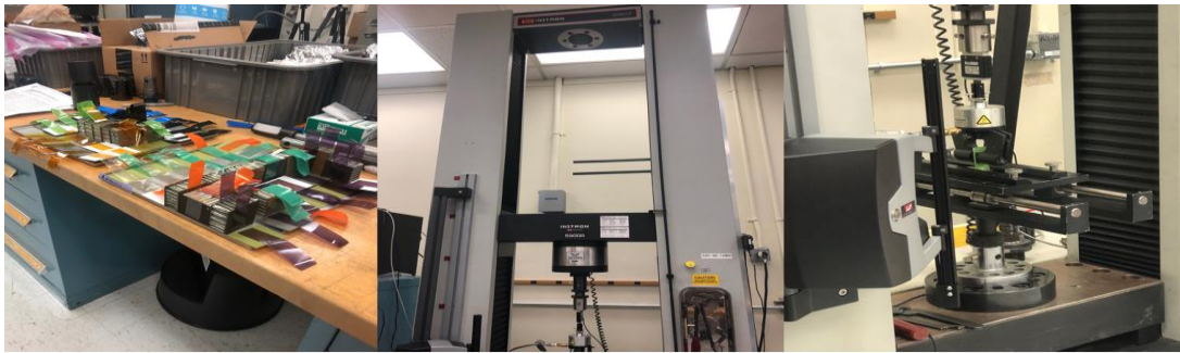
Figure 5: Tapes/coupons samples in mechanical testing room after IOZ departure (left). The 4507 Instron before peel test with sample already prepped (middle and right).
