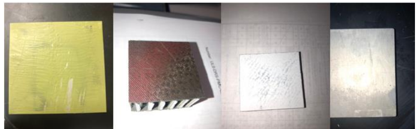
Figure 4. Coupons (left to right: Koropon, composite-rough, Elimstat on Vamac, and titanium) after several tests that are slightly damaged/discolored by cleaning.
