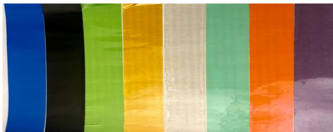
Figure 1. Tapes (from left to right): 3M 471, 3M 481, FB-1R, KPT-1, 3M 5490, 3M 851, CHR 734, BA 12989
