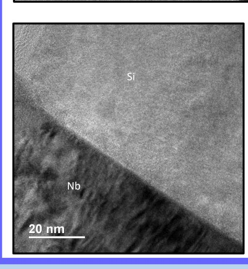
After: TEM image showing Nb-Si interface of **CPW** resonator which R12C1, underwent modified Nb liftoff process. Here the contact is sharp with evidence amorphous layers.
