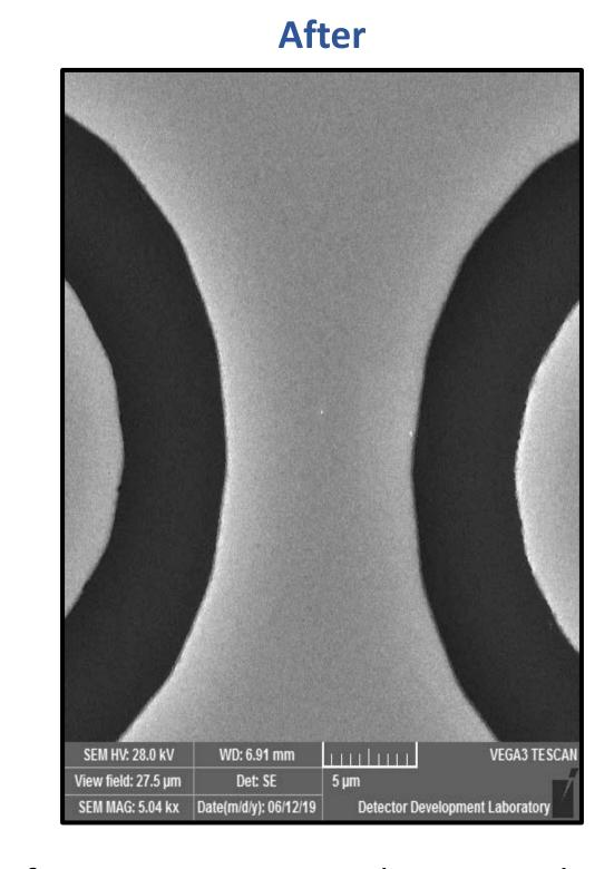
After successive oxidation and etch cycles the extended tails are and the resulting removed significantly measured Q is (more than 10X) higher. See table below.
