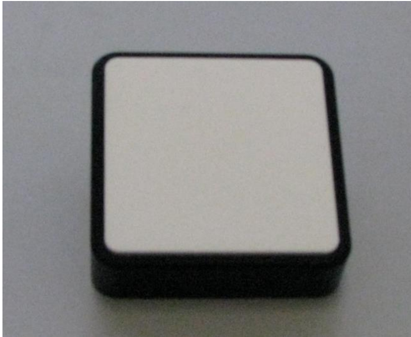
Spectralon: A NIST standard for reflectance, is composed of a pressed powder.
