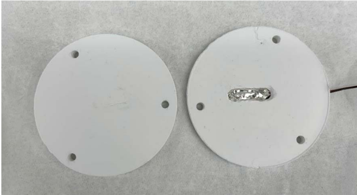
Y_2O_3 samples with temperature sensor
