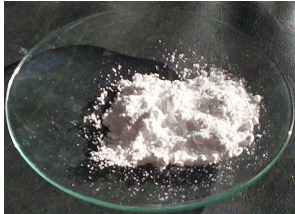
Titanium Dioxide Powder: 0.25 micron particles used as the basis for white paint.
