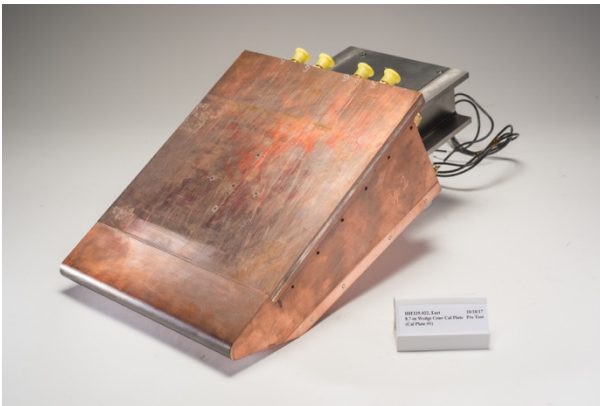
(a) wedge model, water-cooled calibration plate
