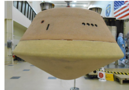
OSIRIS-REx forebody TPS. (~0.8m diameter)
