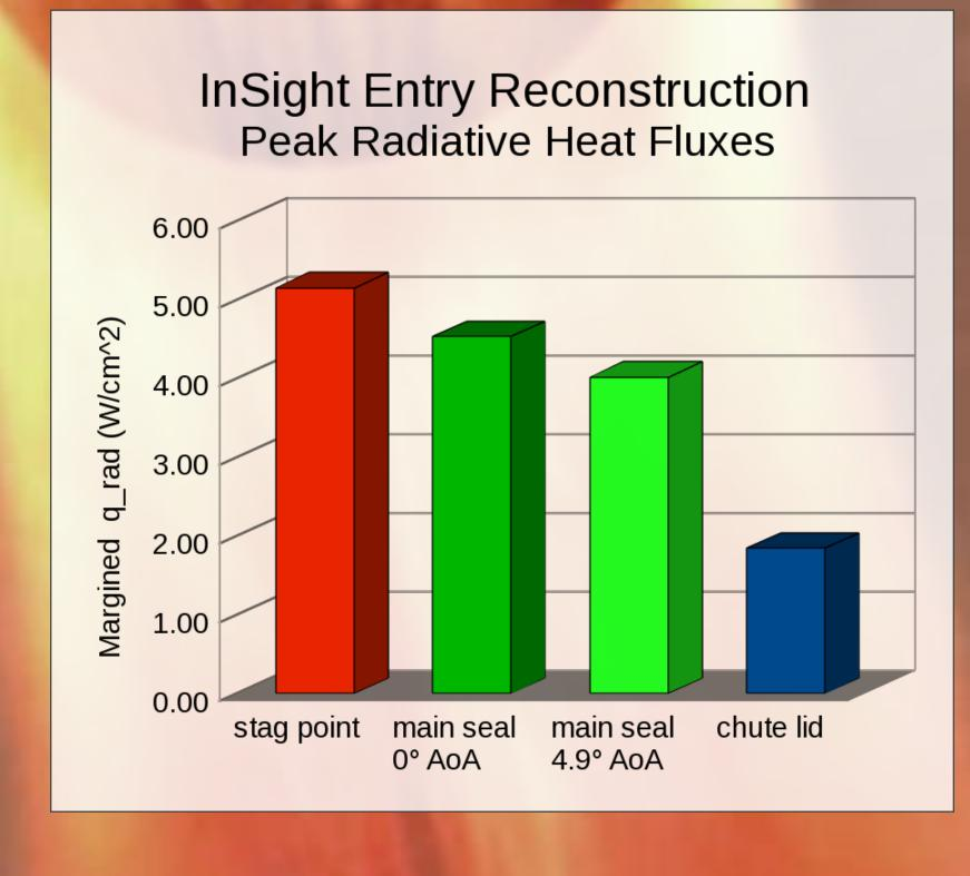
Comparison of radiative flux at main seal for both 0° and 4.9° AoA indicates little impact of flight dynamics on main seal environment. Stagnation point and chute lid are even less sensitive to AoA due to view factor.
