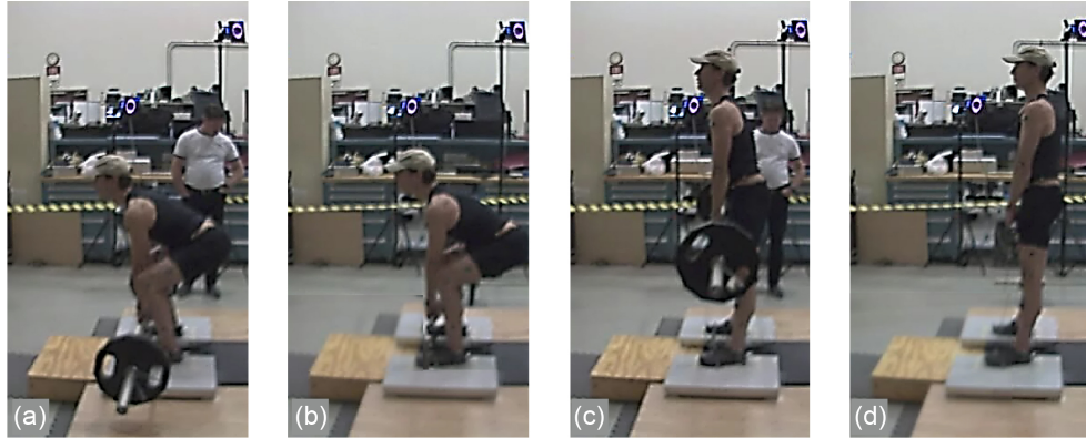
Figure 12.—Comparison of subject posture during deadlift. (a) At bottom of movement for free weight. (b) At bottom of movement for T-bar on Hybrid Ultimate Lifting Kit (HULK). (c) At top of movement for free weight. (d) At top of movement for T-bar on HULK.
