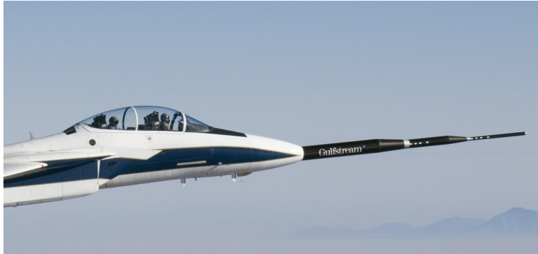
Fig. 1 Gulfstream QuietSpike TM in flight [NASA image].
