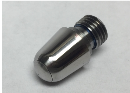
Fig. 20 Nosetip of R_N = 5.08 mm with 210 equally spaced 15 \mu\text{m} cubical roughness elements that were laser-machined circumferentially at 45^\circ from the apex of the spherical tip.
