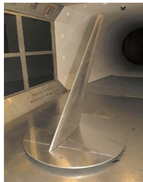
Figure 2. Photographs of 13.3% scale CRM65 semispan wing installed in ONERA F1 wind-tunnel test section (top) and 8.9% scale CRM65 semispan wing installed in WSU wind-tunnel test section (bottom).
