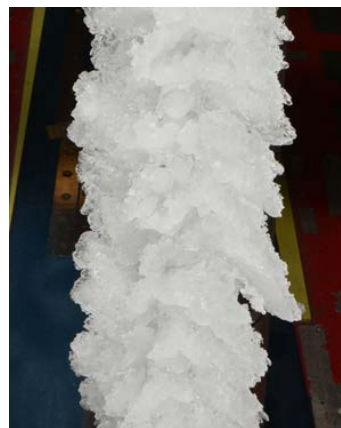
Figure 3. Photographs of WB33 ice accretion on Inboard (top), Midspan (middle) and Outboard (bottom) models.
