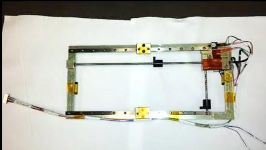
Flight AMT with thermocouples attached for testing
