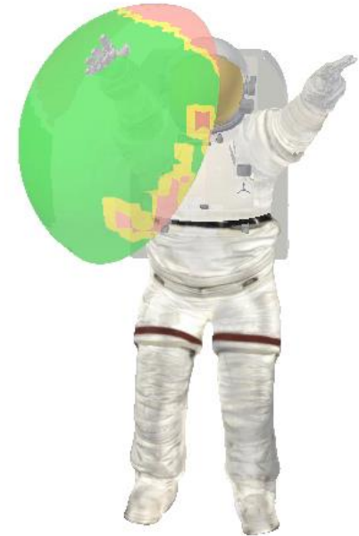
EMU mechanical reach envelope with intra-suit interferences highlighted
