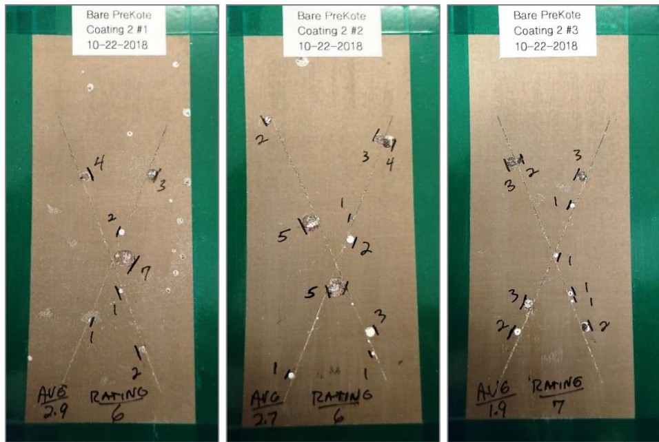
Figure 18. Coating 2 on AA2024-T3 panel with PreKote pretreatment after 2000 hours of salt fog exposure showing ASTM D1654 ratings with an average of 6.
