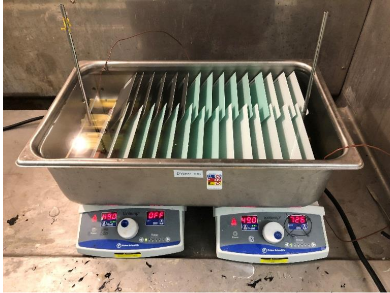
Figure 8. DI water immersion tank for MIL-PRF-23377 water resistance performance test.
