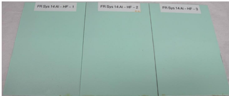
Figure 47. Coating 14 on Alodine pretreated AA2024-T3 panels after MIL-PRF-23377 hydraulic fluid resistance testing.
