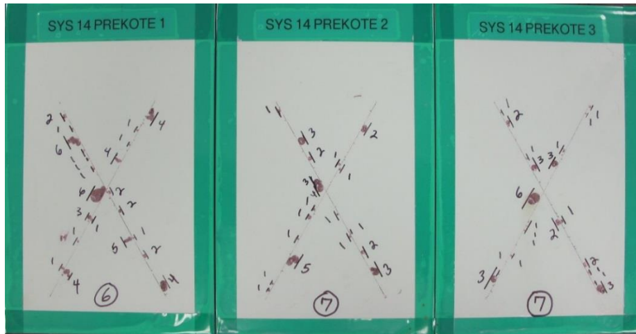
Figure 35. Coating 14 on AA2024-T3 test panels, with PreKote pretreatment, after 2000 hours of salt fog exposure with an average ASTM D1654 rating of 7.
