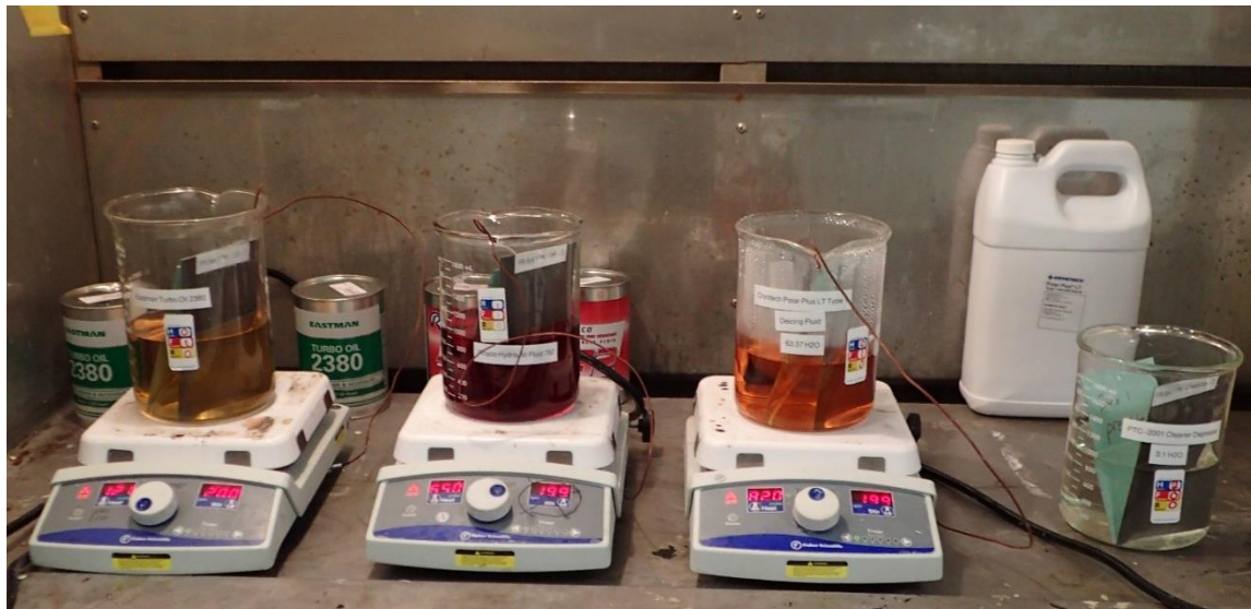
Figure 11. Experimental set up used for MIL-PRF-23377 lubricating oil and hydraulic fluid resistance testing.
