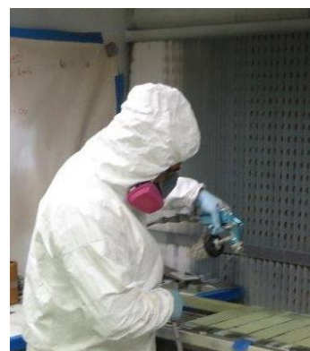
Figure 49. HVLP primer coating application.
