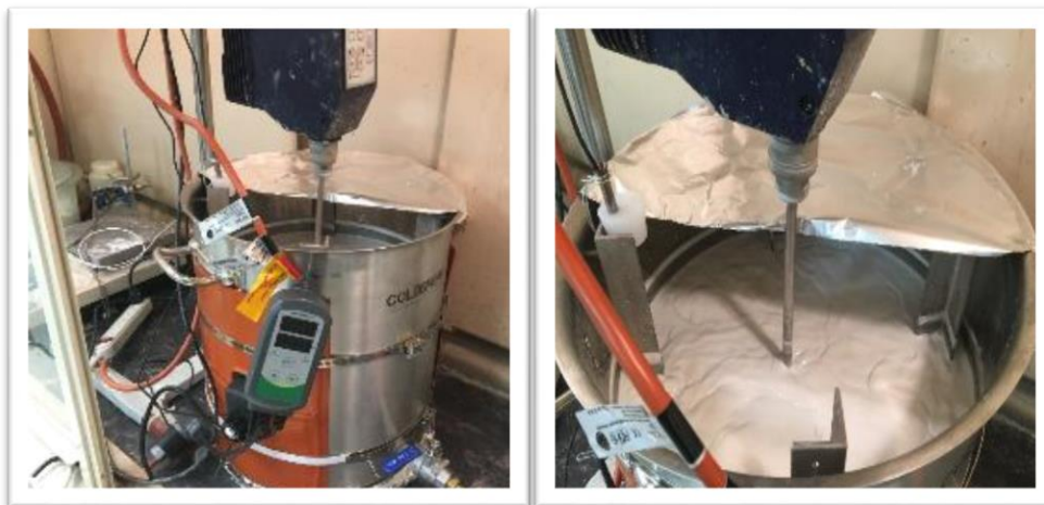
Figure 14. Setup for scaled-up synthesis of 4 kg of 2-MBT micro particle.
