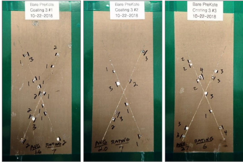
Figure 19. Coating 3 on AA2024-T3 panel with PreKote pretreatment after 2000 hours of salt fog exposure showing ASTM D1654 ratings with an average of 7.
