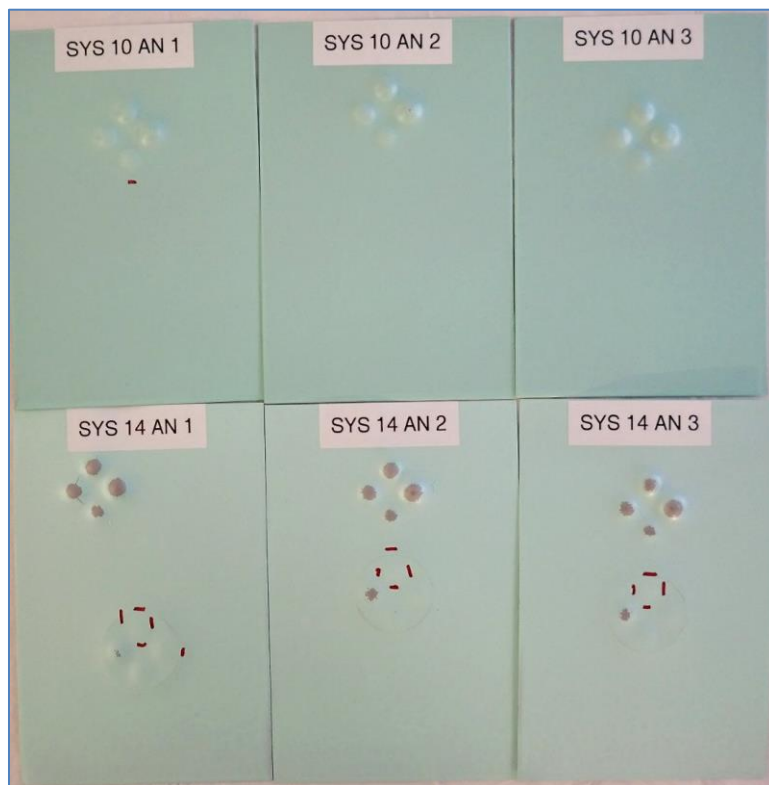
Figure 45. Flexibility test panels for coating 10 test panels (top) and coating 14 test panels (bottom).
