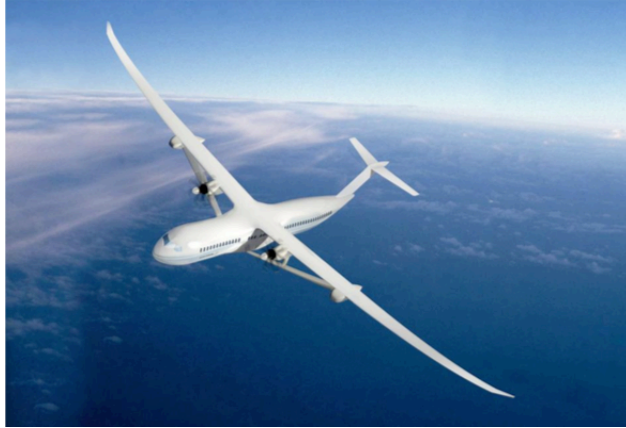
Figure 1. Boeing SUGAR Transonic Truss-Braced Wing (TTBW) Aircraft Concept
