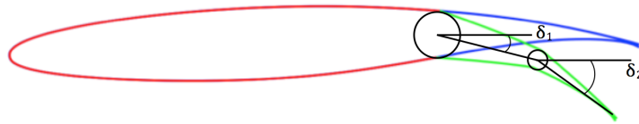
Figure 10: Deflection angles of VCCTEF chord-wise flaps.
